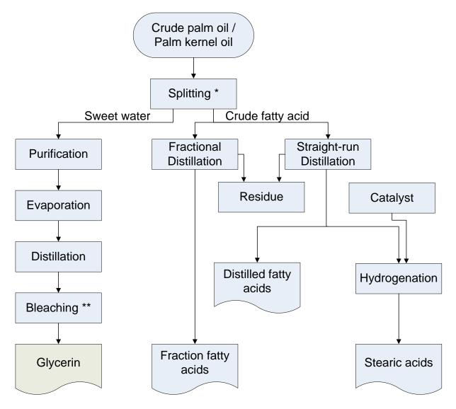
\* Using high temperature steam fractionation
